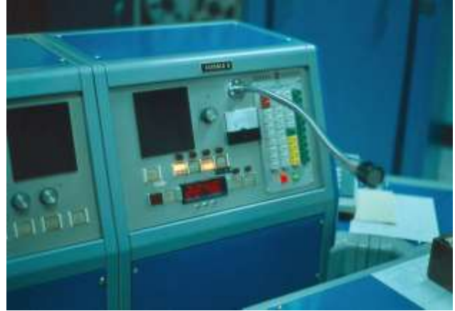
City Fire dispatch console showing buttons for setting off the knockout tones.
